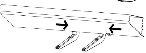
4. Slide the Mounting Brackets behind the rocker panel and in front of the DEF tank as indicated. The left Mounting Bracket will only move so far due to interference from an inner brace.
