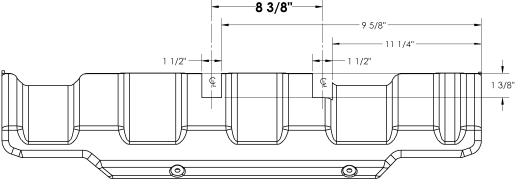
2. With the dimension provided, cut the two slots out on this cover. It is recommended to use a Dremel or similar tool to grind these slots. Cutting with a saw may crack the plastic.
