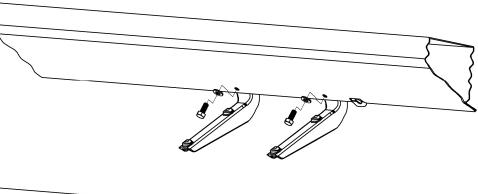
7. Once again, remove the DEF tank cover. Also remove the Step Casting from the Mounting Brackets. Move the Mounting Brackets to the side. Center punch the center of each cross-hair mark. Drill out the centers with a 1/8" drill bit and then go back and drill out the holes with a 11/32" drill bit. Remove all burrs. Refer to Step 8 on Page 2 for installing 5/16" hardware.
