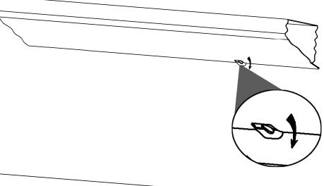
3. Bend the protruding tab down to allow the front Mounting Bracket to be in its proper position. Channel Locks or similar tool will make this easier.
