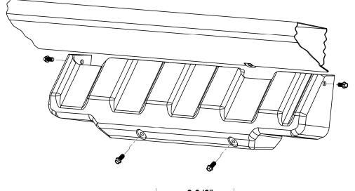
1. Under the passenger front door, remove the black DEF plastic tank cover from your vehicle. You will need a 10mm socket to remove the four bolts. Keep these bolts for reinstallation.
