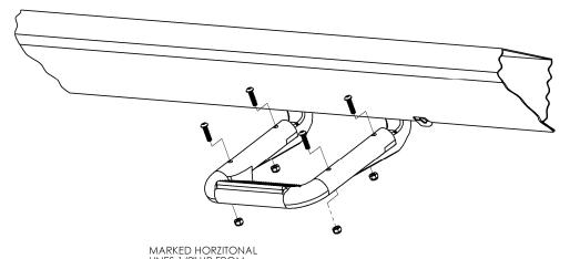
5. Place the Step Casting on the Mounting Brackets. Take the ¼" hardware provided and hand tighten the hardware.
