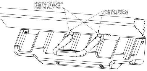
6. Reinstall the DEF tank cover. Slide the Mounting Bracket/Step Casting assembly so that the back of the Mounting Brackets line up with the slots in the DEF tank cover. Mark the lines on the vehicle's body metal as indicated on the drawing. Make sure the 8 3/8" vertical lines are on center with the Mounting Brackets.
