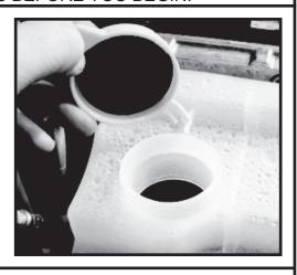
Step 2. Install the retainer wire around the neck of the tank first. Install the new billet cap onto the reservoir.
