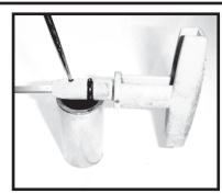
Step 2. Install the small sleeve over the end of the dipstick. Insert the dipstick and sleeve into the handle. Align the hole in the dipstick, sleeve and handle.
