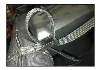
11. Innermost polyester straps on Top Net, toward back of vehicle, include (2) plastic strap adusters sewn onto bottow of Top Net. Wrap nylon straps around top of roll bar, into strap adjusters, then pull tight. Complete Cargo Net System installation.
