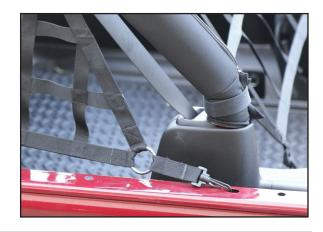
8. It is recommended to attach front plastic hook of Side Nets to child car seat anchors.
