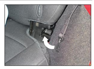
9. OPTIONAL: lift carpet between rear seat and side fender, use supplied footman loops and a marker to mark screw locations. Drill pilot holes at marked locations using a 9/64" drill bit. Attach supplied footman loop using Sheet Metal Screws placing plastic spacers between footman loop and sheet metal. Replace carpet, then cut carpet above footman loop using utility knife. Attach plastic hook to installed footman loop.
