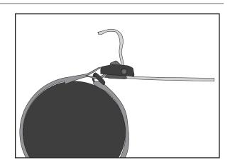
4. Install Side Nets by attaching metal rings to roll bar using Long No-Velcro Straps. Install Top Net corner metal rings by attaching one Long No-Velcro Strap to roll bar and one Short No-Velcro Strap to factory footman loop. Attach Top Net center metal ring to factory footman loop using Short No-Velcro Strap. Attach Back Net metal rings to roll bar using Long No-Velcro Straps.
