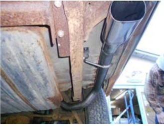
3) Place the left side exit pipe **#86148** up into place and connect the hanger at the rear of the pipe to the rubber mount installed in step 1 above. Slide the hanger into the rubber mount until about  $\frac{3}{4}$ " of the wire hanger sticks out from the rear of the rubber mount. Repeat this step on the right side of the vehicle with exit pipe **#86147**.
