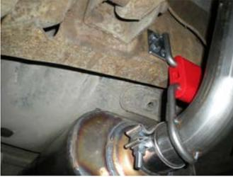
4) Place a red **HA168** hanger onto the hanger of the left over-axle pipe **#86144**. Also place a provided clamp onto the expanded end of the pipe. Then place the pipe up into position over the rear axle and connect to the exit pipe. Be sure that the two pipes are fully slid together and then slide the rubber hanger onto the cross member mount installed in step 2 above. Tighten the clamp enough to hold but still allow for adjustment. Repeat this step with the right over-axle pipe **#86143**.
