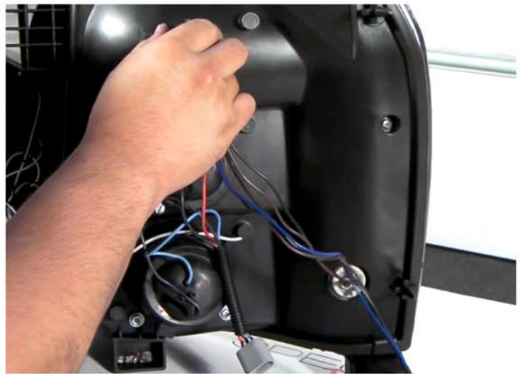
10. Connect all the connectors and harness to new headlight Please see the "Halo and L.E.D installation instructions" If your headlights don't have HALO or L.E.D. You can skip
