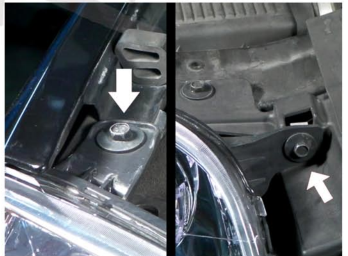
4. Remove two headlight bolts
