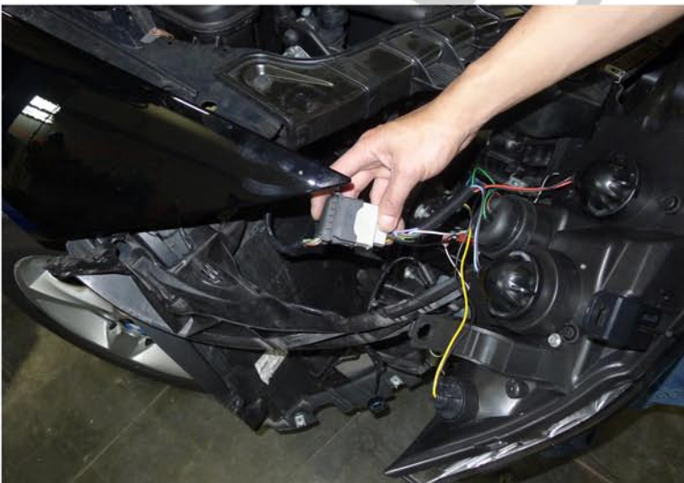
21. Connect the headlight harness to the new headlight Please see the Halo and L.E.D installation instructions. If your headlights don't have HALO or L.E.D. you can skip it
