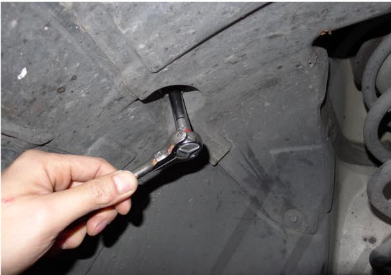
13. Remove the (2) 8mm screws
