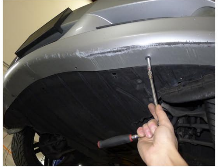
38. Tighten the (3) 10mm bolts
