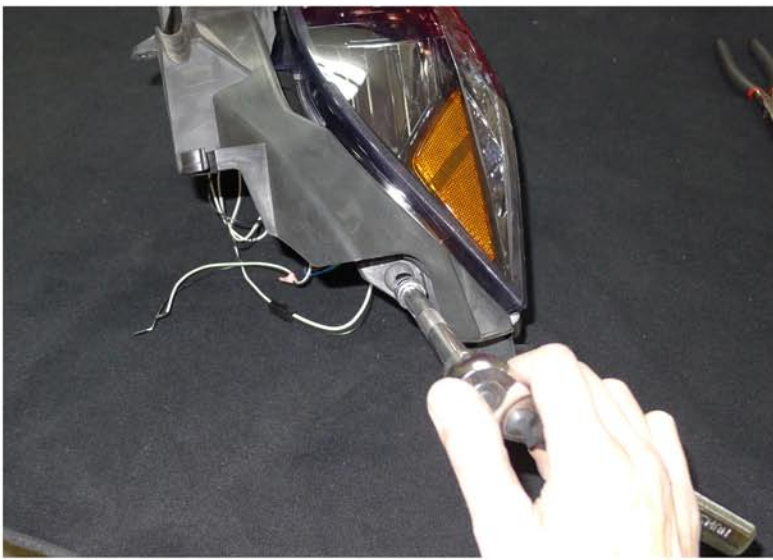
23. Tighten the T30 bolt
