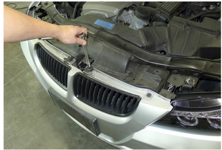
34. Tighten the (4) T30 bolts
