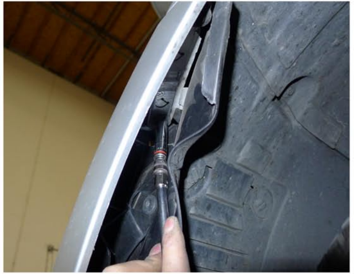
36. Tighten the (2) 8mm screws
