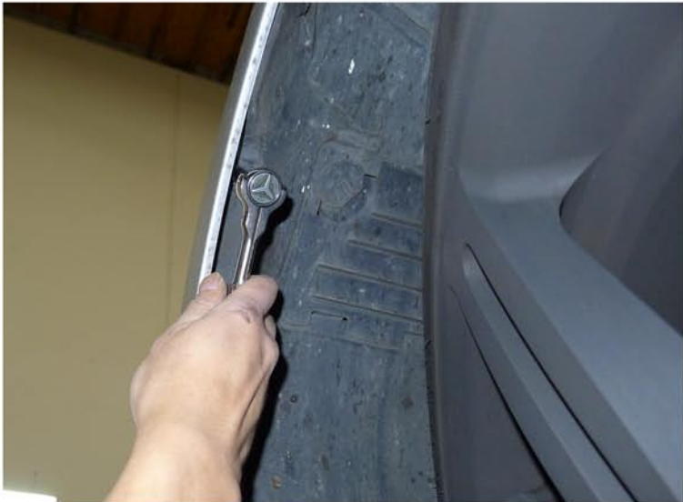
37. Tighten the (2) 8mm screws
