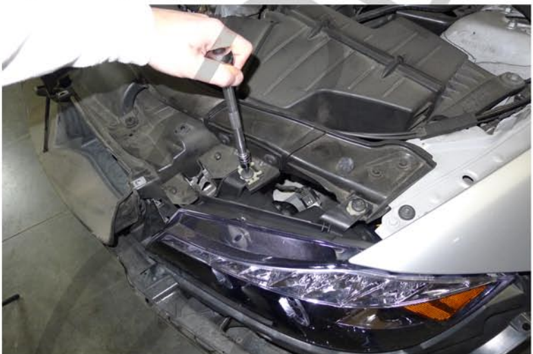
27. Tighten the (2) T30 bolts
