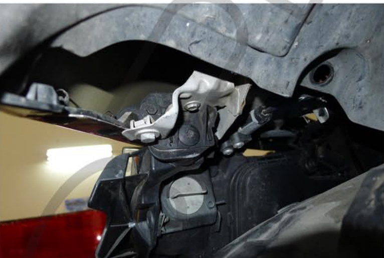
17. Pull the fender liner aside
