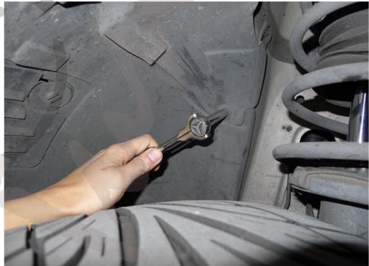
14. Remove the (2) 8mm screws
