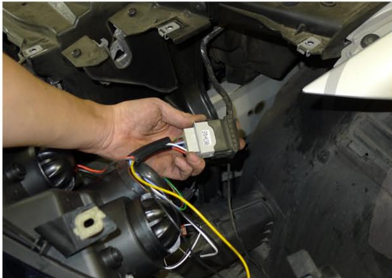
25. Connect the headlight harness to the new headlight Please see the Halo and L.E.D installation instructions If your headlights don't have HALO or L.E.D. You can skip it
