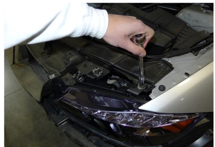
28. Tighten the (2) T30 bolts
