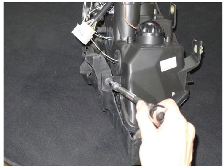
24. Tighten the T30 bolt
