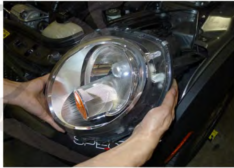
8. Remove the headlight
