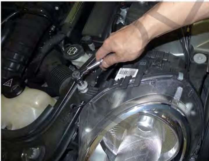
3. Remove the (2) 10mm bolts
