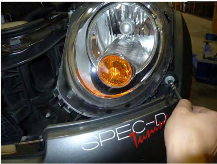
5. Remove the (2) 10mm bolts
