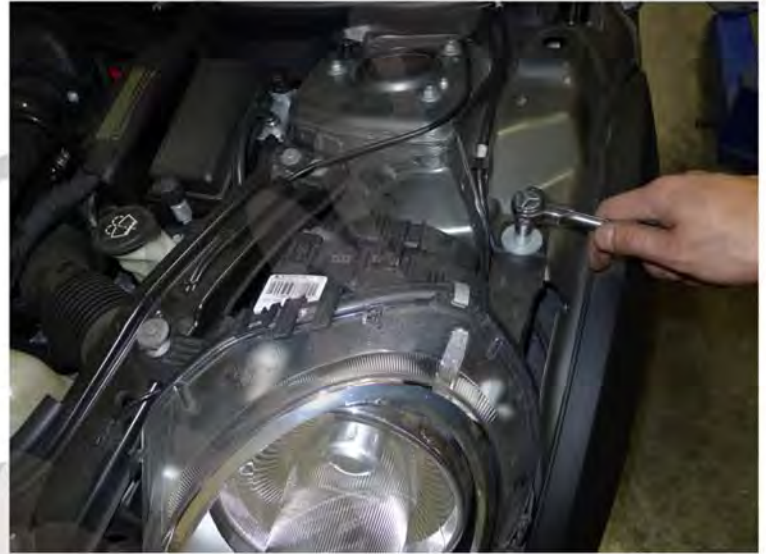
2. Remove the (2) 10mm bolts
