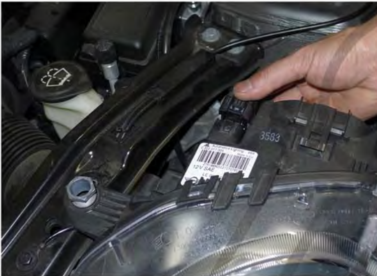
7. Disconnect the headlight harness
