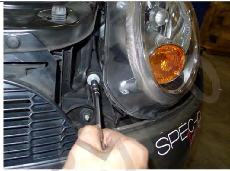
6. Remove the (2) 10mm bolts
