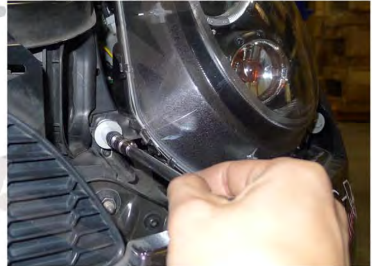
14. Tighten the (2) 10mm bolts
