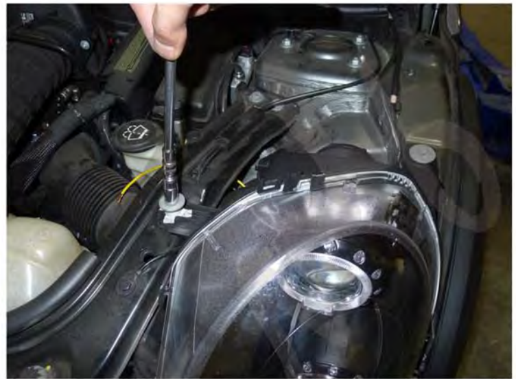
12. Tighten the (2) 10mm bolts
