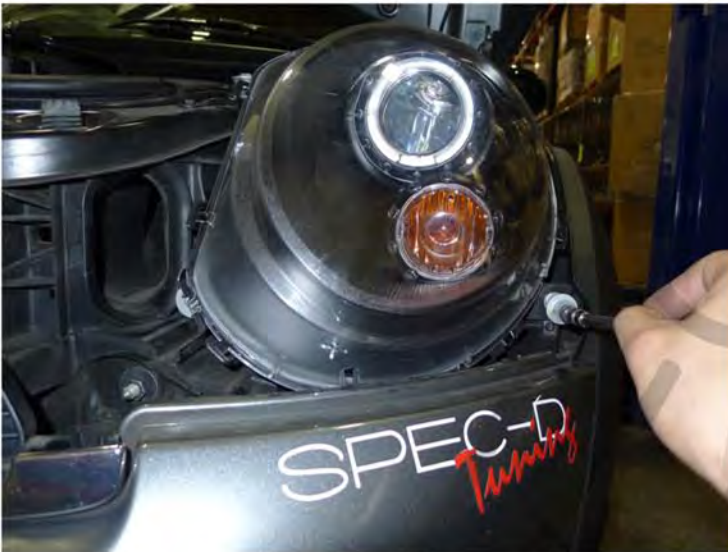
13. Tighten the (2) 10mm bolts
