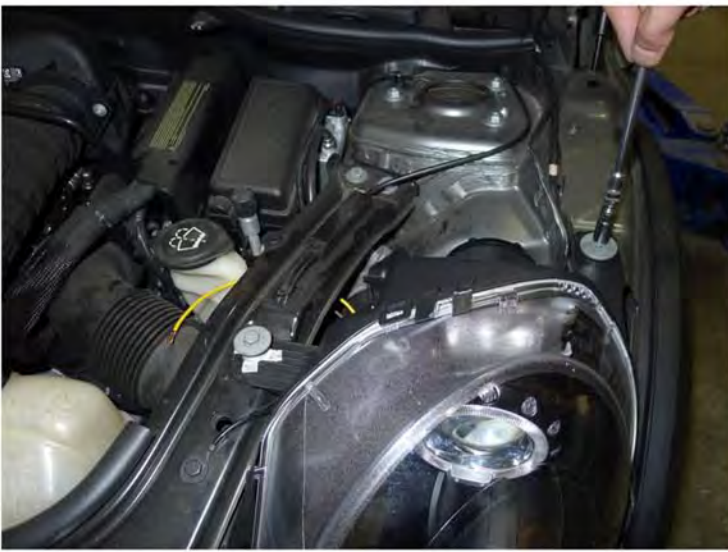
11. Tighten the (2) 10mm bolts
