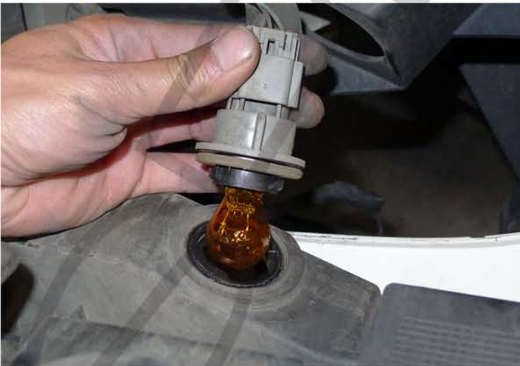
9. Remove the turn signal light socket
