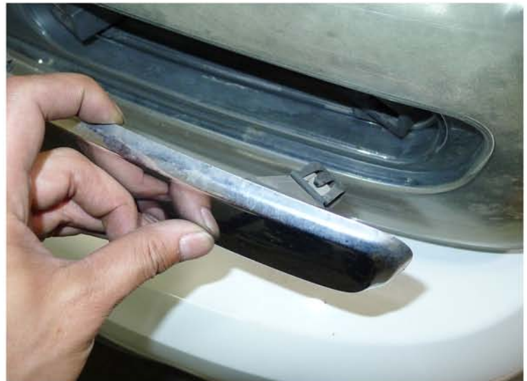
4. Release the front grill retaining clips
