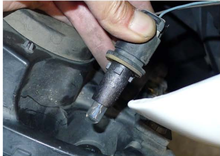
10. Remove the parking light socket
