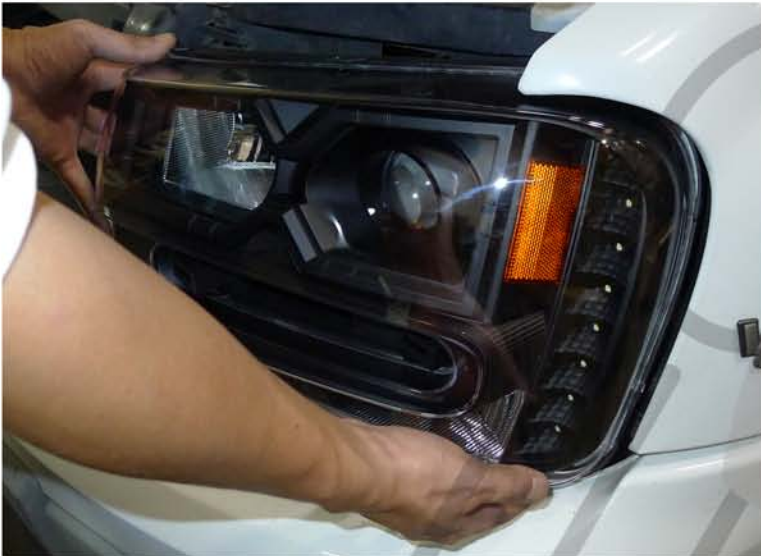
13. Place the new headlight into the position
