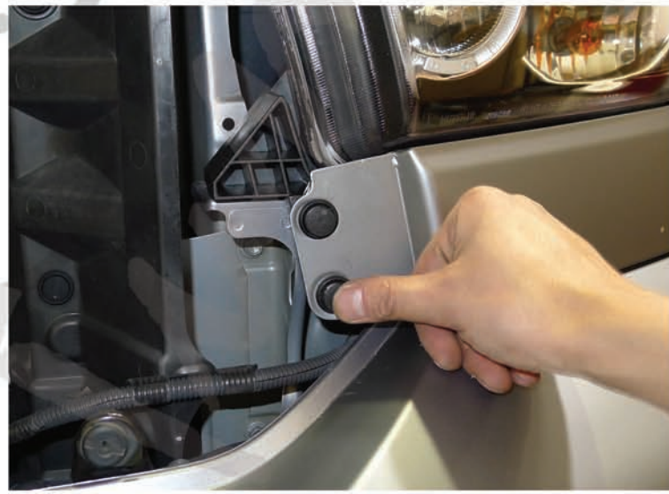
14. Replace the (2) plastic clips Please repeat the steps from 1 to 14 for the opposite side
