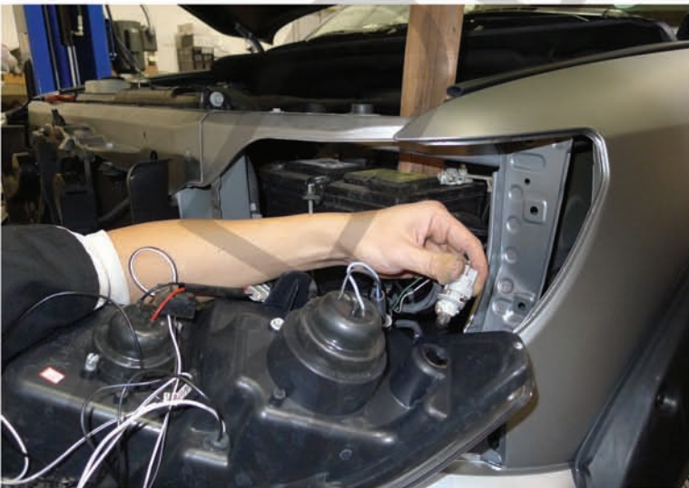
9. Connect the headlight harness to the new headlight Please see the " Halo and L. E. D. headlights installation instructions" If your headlights don't have Halo and L. E. D. You can skip the installation instruction.
