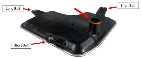
9. Install the ATS Billet Extended Pickup Tube as shown.
