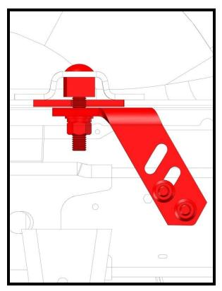
If needed, the lower portion of this hat channel can be removed for easier installation of the "L" bracket and mounting hardware.
