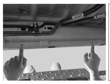
3. With both holes marked, center punch both marks and drill out with the 1/8" drill bit followed by the 5/16" drill bit. Try to clean out burs as best as possible. Be careful not to drill into plastic trim. The step and brackets will need to be disassembled for the next step.
