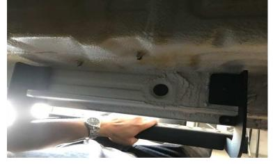
2. With step assembled, place step in the desired location avoiding any bumps or indents to allow both brackets to be parallel to each other. With a marker mark both holes for the 5/16" mounting hardware; top holes do not need to be marked. Excess caulking will have to be cut to allow better fitment of brackets.
