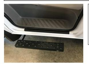
6. Re-install your step and with the 3/16" Allen wrench and  $\frac{1}{2}$ " socket fully tighten all four button head screws.
