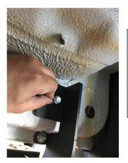
7. Fully tighten both 5/16" hex bolts to pinch weld. Finally with a 3/8" socket install the #14 self-tapping screws to both brackets and be careful not to over tighten them. Your step is now fully installed follow the same procedure for other side.
