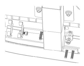
4. Take one of the "C" Brackets and slide it on to the shorter carriage bolt with a washer and nylon lock nut and only hand-tighten. Place two additional longer carriage bolts through the two holes at the bottom of the "C" Bracket. See diagram.
