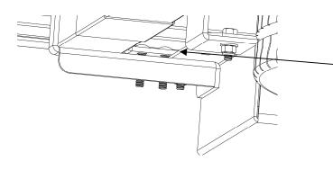
9. Make sure the feet of the "C" Brackets from Step 4, on both sides, are on top of the flange of the black powder coated pan.
