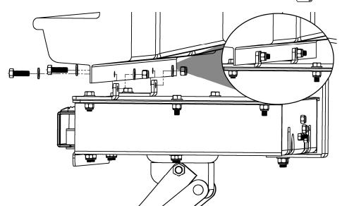
5. Lower the front end of the step down to expose the marked holes. Take a drill motor (a right-angled drill motor will make this easier) with an 11/32" drill bit and drill out the marked holes. Remove all burrs. Lift the step back into position. Take the remaining 5/16" hardware and securely tighten the Front Steel Brackets to the vehicle.
