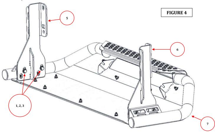
**Step-6** With assistance align and hold the RC3 or RC4 front guard in the desired position on the vehicle, then tighten all OEM and supplied nuts and bolts.
