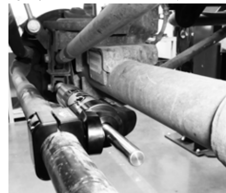
Fig. 2: Stabilizer clamped to tie rod
