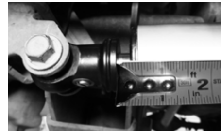
Fig. 1: Eyelet installed and 1/4" of shaft exposed
