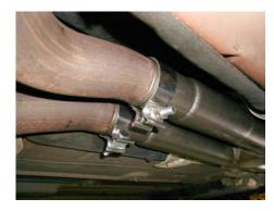
1) Begin the installation by placing a supplied 2-1/2" clamp onto each of the inlets of the X-pipe assembly **#26559M.** Then, place the X-pipe onto the back of the stock head pipes (the embossed Hurst H will be facing the ground). Level and center the assembly in the drive line tunnel and support with a stand. Tighten the two clamps enough to hold, but still allow for adjustment.
