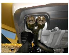
3) Place a supplied clamp onto the left muffler outlet. Place the left tailpipe #26564M into position and starting from the rear, connect the hangers on the tailpipe to the rubber mounts on the vehicle. Slide the tailpipe fully into the muffler outlet. Adjust the tailpipe so that the stainless tip is level and centered in the bumper cut-out. Tighten clamp enough to hold, but still allow for adjustment. Repeat this step for right tailpipe #26563M.
