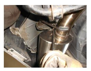
3) Place a 3" clamp onto the inlet pipe of the left muffler assembly **#3510005-414**. Place the muffler up into position and onto the left over-axle pipe and then connect the rear hanger on the muffler to the rubber mount on the vehicle. Secure the double hanger mount back into position on the frame using the factory bolts. Repeat this step on the right side of the vehicle with muffler assembly **#3510005-415**.
