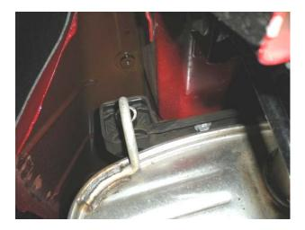
4) There are three hangers on each muffler, two in the front and one in the rear. Separate the rear hanger rods from the rubber mounts first then slide the mufflers forward and out of the front mounts. A spray lubricant will help the hangers to slip out. Using a 13mm socket, remove the bolts securing the double hanger mounts at the front of each muffler from the frame on the left and right side of the vehicle. Place the mounts onto the front hangers of the corresponding Hurst muffler.
