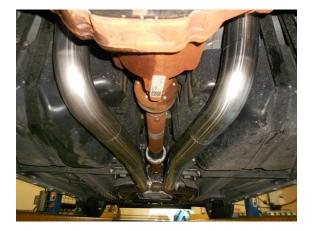
2) Place the left over-axle pipe **#26582H** into position over the rear axle and support with a stand. Then slide the front of the pipe into the clamp installed on the back of the factory H-pipe. Slide the pipe fully on and tighten the band clamp nuts enough to hold, but still allow for adjustment. Be sure that the over-axle pipe is fully forward. Repeat this step on the right side of the vehicle with pipe **#26583H**. See photos above.
