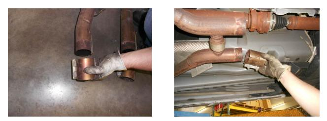
1) Remove the factory band clamps from the original over-axle pipes and place them onto the back of the factory H-pipe.
