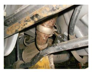
2) Loosen the 13mm bolts on the clamped connections between the mufflers and the over-axle pipes. The bolts need to be backed out to the end of the threads in order to open the clamp enough to allow the flared ball connection of the inlet pipe to be removed. Separate the over-axle pipes from the mufflers.
