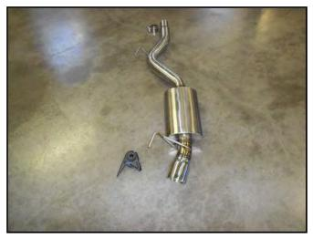
1) Place the new Hurst muffler units next to the factory units and swap the front and rear hanger mounts from the stock mufflers to the Hurst assemblies. Also, place a provided 2-1/4" clamp onto the inlet of each assembly. Tighten the clamp just enough to hold in place.
