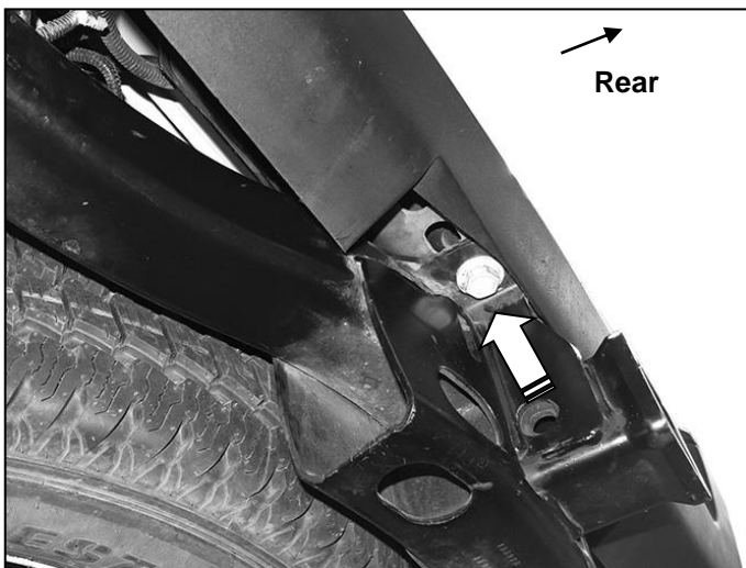
(Fig 1) Factory bumper may be attached to top of tow hitch. Remove factory hex bolts as required.
