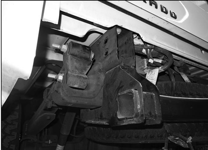
(Fig 3) End of frame once factory bumper is removed
