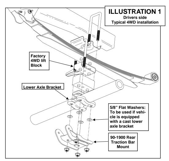
NOTE: If installing this kit while the vehicle is on a lift, be sure to lower it to the ground before installing the front mounts and the traction bars.
