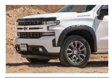
**STEP 9:** Ensure all fixing points are tight and secure and that the rubber seal is flush neatly against the vehicle body. Repeat install steps for the opposite side.
