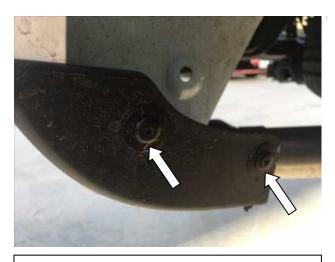
**STEP 14:** Using #15 Torx head screwdriver remove the two botton screws from the rear factory spat. Maintain screws for re-install.
