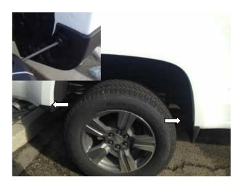
**STEP 8:** Locate the 2 outer screws. Remove the screws using a #15 Torx head screwdriver. Retain screws for installation.
