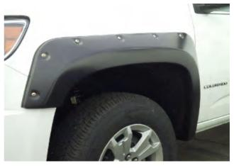
**STEP 6:** Repeat installation method for other side. Double check the front Fender Flares to make sure all bolts are tight and clips are securely fastened.
