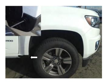
**STEP 2:** Locate the Torx screw at the lower section of the wheel well. Remove the Torx screw using a #15 Torx head screwdriver. Retain the screw for installation.
