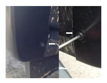
STEP 10: Reinstall the #15Torx head screws.
