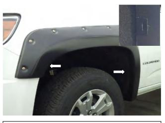
**STEP 4:** Use 2 of the small U-style clips to secure the Fender Flare to the body. Make sure the barb in the clip securely attaches in the slot on the Fender Flare.
