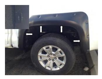
**STEP 9:** Place the Fender Flare onto the vehicle and fit into the correct position following the contours of the body. Use 4 of the U-style clips to secure the Fender Flare to the body. Make sure the barb in the clip securely attaches in the slot on the Fender Flare.
