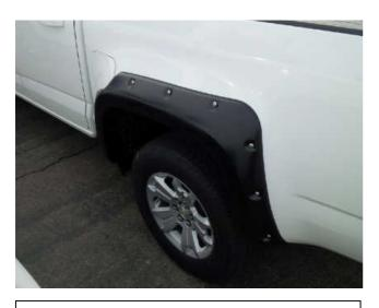
**STEP 11:** Repeat installation method for other side. Double check the front Fender Flares to make sure all bolts are tight and clips are securely fastened. Your installation is now complete. Do not use abrasive cleaners.
