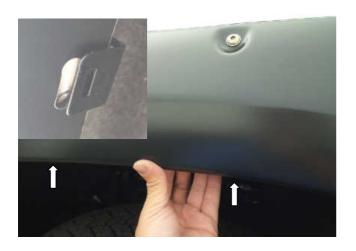
**STEP 3:** Place the Fender Flare onto the vehicle and fit into the correct position following the contours of the body. Locate the 2 mounting slots on the top of the fender flare. Use 2 of the large U-style clips (indicated with an X on the clip) to attach the fender flare. Make sure the barb in the clip securely attaches in the slot on the Fender Flare.
