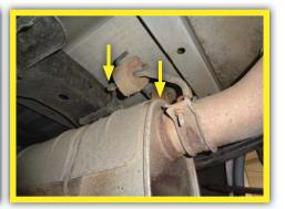
5. Remove muffler and set aside.
