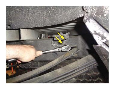
14. Place hanger (503HA) onto vehicle frame then reinstall factory bolts (x2) (removed step 13). Install isolator (HA168) onto hanger.
