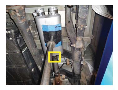
Place right tailpipe (26733S) into passenger side muffler outlet. Insert both wire hangers into stock mounts to complete connection. Tighten clamp just enough to allow for adjustment.
