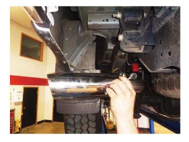
18. Place **tip (ST462)** onto side or rear exit pipe. Tighten clamp just enough to allow for adjustment.
