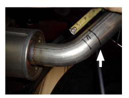
4. Cut driver and passenger side tailpipes off at marked lines and remove them from vehicle.
