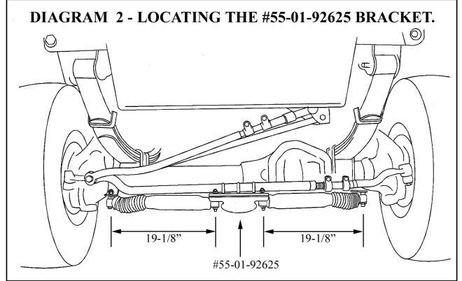
position the bracket so that the distance between the stabilizer mounting studs on the axle and the studs on the "02" bracket is 19-1/8". Tighten (26).
