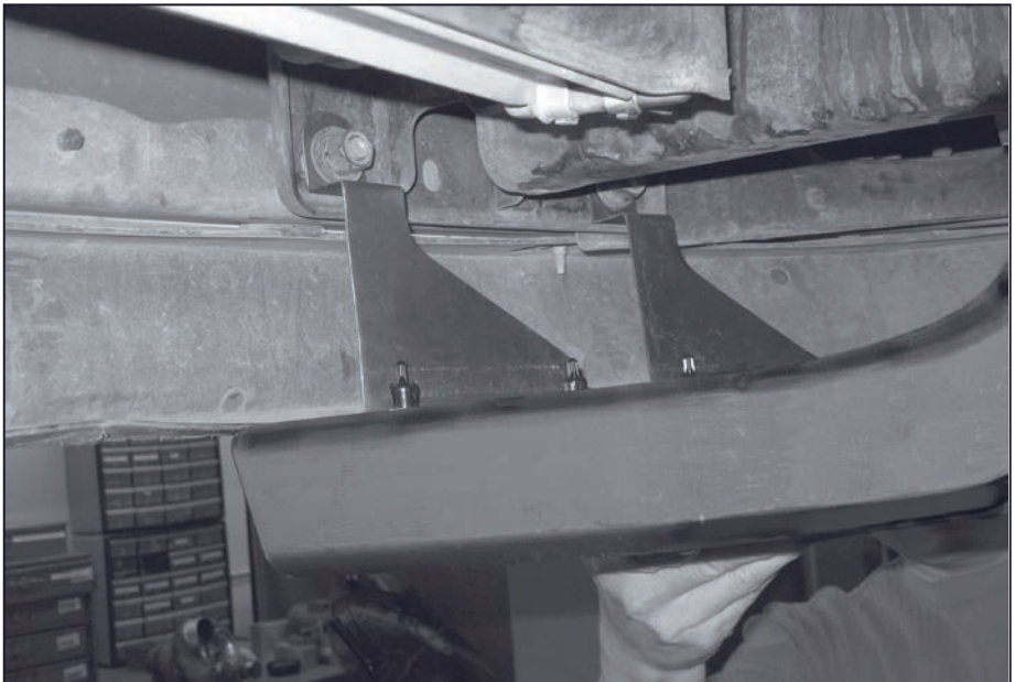
Figure 6 Install Super-Scoop support brackets over factory bolts
