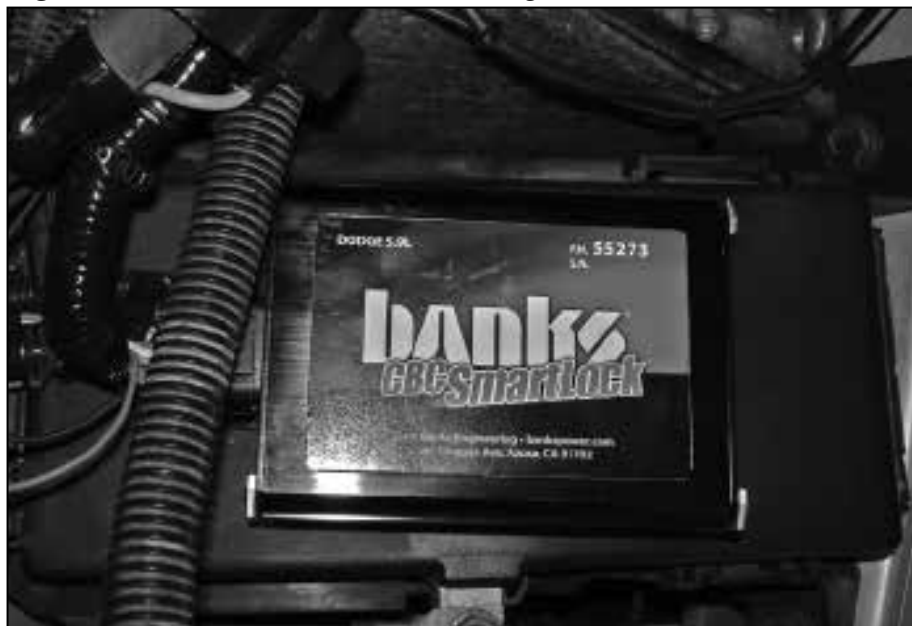
Figure 32 All Models CBC Smartlock Mounting Location
