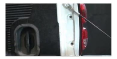
Located here are the two Torx 25mm bolts that will need to be removed in order to get the OEM tail light assembly separated from the body.
