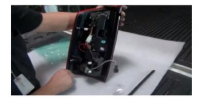
4) On the back of the new Spyder tail light is a small grey socket on the bottom of the assembly. Turn this socket and remove it as you will need to transfer over the stock reverse bulb into this harness. Once the bulb is in place, install back into the unit and lock into place.
