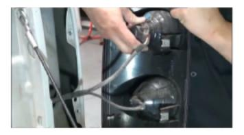
3) Once you've removed the bolt, gently pry the assmbly free. On the back of your tail light you will have 2 bulb connectors; one for brake (top) and one for reverse (bottom), remove these by turning the bulb counter clockwise. Set OEM assembly aside.
