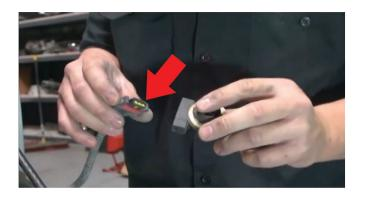
6) Next, once the brake bulb has been removed you can now separate the brake bulb socket from the harness. This will enable you to use the LED harness provided with the Spyder tail light.
