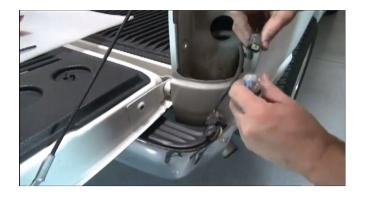
5) In order to remove the bulbs, gently pull on the bulb until it it pops free of the harness as shown above. Once the reverse bulb has been removed, you may now put this bulb in the lower harness connector on the spyder tail light. (See Fig. 4)
