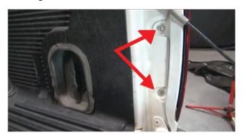
10) Place the tail light unit back into place, line up the mounting holes and replace with the phillips screws. Tighten both down, and you're done!
