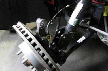
Support the lower control arm with a floor jack, remove the lower strut mounting bolts and lower the floor jack to remove the strut assembly.
