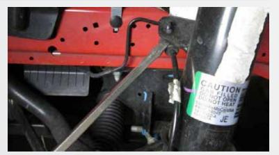
Remove the strut tower brace is applicable. Starting with either driver side or passenger side remove the wheel. Disconnect the brake line bracket and detach the ABS sensor wire from the strut body.
