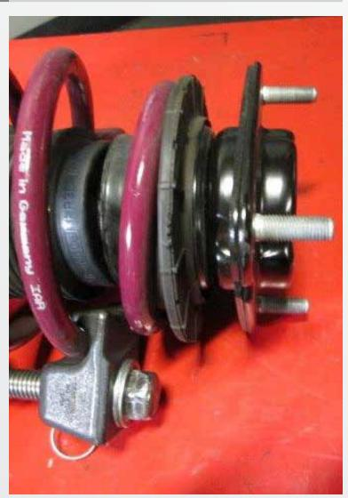
With a spring compressor, slowly depress the spring, then remove the upper strut retaining nut, then remove the upper strut mount assembly from the strut shaft. NOTE! Recommend the use of an impact gun.
