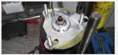
Install the Camber/Caster Assembly to the supplied Ford Strut Tower Pivot Assembly.
