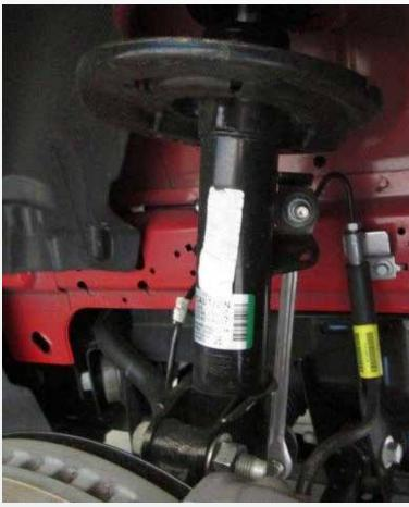
Remove the sway bar end link from the strut, then loosen but do not remove the strut mounting bolts.
