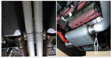
You will need to rotate the BBK Under Axle Pipe one way or the other to get the muffler in place once in place tighten down the 3" barrel clamp and the band clamp at the inlet tube of the muffler.
