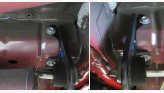
Remove the 2 bolts on the driver side and passenger side that hold the muffler mount to the chassis.
