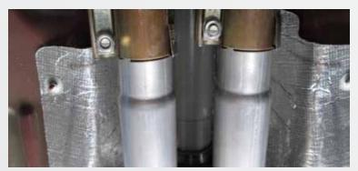
With the BBK Cat Back System install on the vehicle. Level out the BBK X-Pipe adapter and push it all the way forward towards the front of the vehicle and tighten down the stock 2 1/2" barrel clamps.
