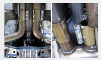
Loosen the 2 barrel clamps at the front of the resonator that connects it to the mid pipes of the exhaust.
