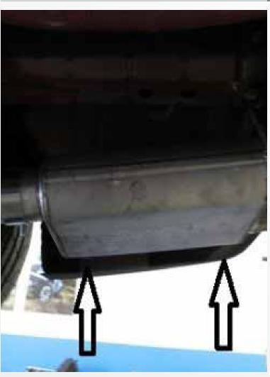
Level and straighten out the muffler using a muffler stand or jack stand to hold it in place.
