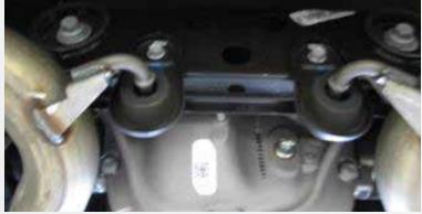
Remove the 2 bolts on the exhaust mounts located on the rear differential cross member and unhook them from the chassis.
