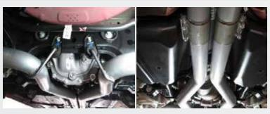
Install the 2 rear differential cross member mounts onto the BBK Under-Axle pipes. Using the (2) 3" couple supplied in the kit slide them onto the BBK X-Pipe adapter.
