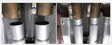
Install the BBK X-Pipe adapter to the stock mid pipes of the exhaust using the stock barrel clamps.
