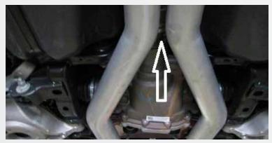
NOTE! Be sure to check the clearance in between the BBK Under Axle Pipes and the drive shaft CV joint when rotating and adjusting the pipes.
