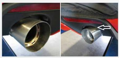
Slide the 3 "band clamp onto t the exhaust tip, then slide the exhaust tip onto the outlet tube of the muffler.
