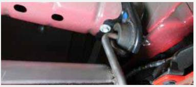
Slide the muffler over the inlet pipe, then lift the muffler into place and attach the mount to the body, install the 2 bolts that hold the mount to the body and tighten them down.
