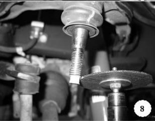
is recommended that when you remove the lower portion of the stud you leave at least 1/16" of the stud extended out from the nut. It is also recommended that once the stud is trimmed off you use a chisel or punch to score the edge of the threads to prevent any possibility of the nut coming loose (illustration 18).
