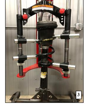
NOTE: If a half inch increment lift height is desired, please add one 25003-075 ring or 7.5mm equivalent to the shock from the next lowest increment from the table below.
