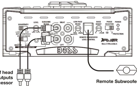
To Audio Outputs of head unit or Subwoofer outputs of a signal processor
