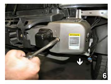
Using the 10MM socket to remove one (1) metric bolt. Do this to both sides of the vehicle. Set metric bolts aside to be reinstalled later. Remove the tow hook assembly with the 12MM socket. The tow hooks will **NOT** be reinstalled.
