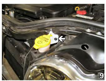
Remove a rivet from the reservoir spout with the diagonal cutters, pull reservoir down and set aside to be reinstalled later.
