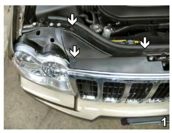
Remove the six (6) pushpins from the black plastic cover on the top side of the fascia. Lift cover up and set aside to be reinstalled later. Pull top of grille forward. Lift up and set aside with pushpins to be reinstalled later.
