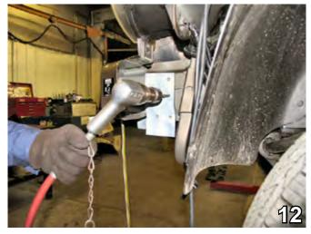
Using the baseplate as a template, drill ALL holes with the 13/32" drill bit. Do this to both sides of the vehicle.
