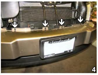
4. Remove four (4) pushpins from the top of the front fascia. Set pushpins aside to be reinstalled later.
