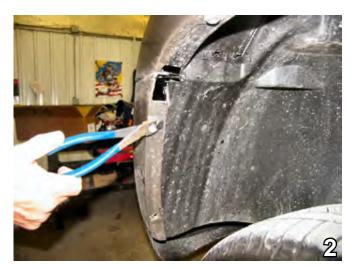
Using the diagonal cutters, remove two (2) rivets from the wheel well cover just forward of the front tires. Do this to both sides of the vehicle. These rivets will be replaced.
