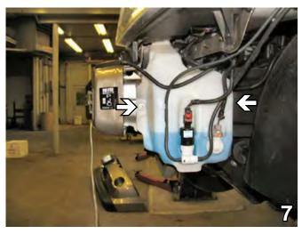
Using the 10MM socket, remove two (2) metric bolts from the washer reservoir on driver's side, unplug the electrical connections, disconnect and plug fluid lines. Set bolts aside to be reinstalled later
