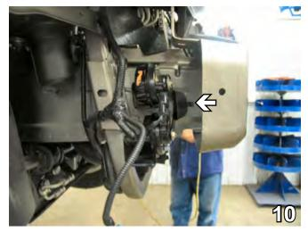
Remove the metric bolt from the horn bracket on the passenger's side with the 13MM socket, unplug the electrical and set horn assembly aside.
