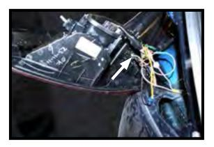
Drill a 1" hole to install the 3 wire automotive socket.
