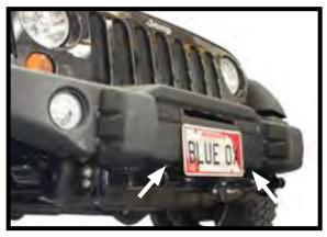
3. If installing a breakaway switch, use a 13MM socket to remove one (1) of the existing bolts on either side of the bumper.
