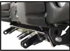
Align the baseplate between the bumper brackets. Insert one (1) of the 1/2"-13 x 1-3/4" hex head bolts and 1/2" lock washers in the bottom hole and tighten securely. Do this on both sides.
