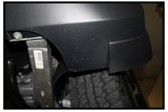
13. Install the new plastic rivets into the underside of the fascia, where the factory rivets were removed.
