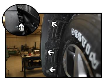
Using a 8MM socket, remove the three (3) screws from the edge of the wheel well.
