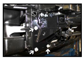
9. Install the baseplate to the vehicle using the three (3) existing extension bolts (white). Install 10MM-1.25 x 40MM bolts with 3/8" flat washers and 10MM lock washers into the lower bumper bolts (gray). Fully tighten all fasteners. Do this on both sides of the vehicle.
