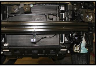
11. **Optional:** If installing a breakaway, screw the breakaway bracket to the bumper at the desired location with the #10-16 x 1" self drilling screw. Attach the breakaway to the bracket with a 1/4"-20 x 3/4" bolt and 1/4"-20 lock nut.
