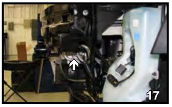
17. Attach the permanent baseplate safety cables to the provided convenience link on the baseplate. The photo above shows the recommended installation of the cables to frame of vehicle. Additional options may interfere with suggested mounting; in this case secure the cables to a solid piece of the frame as described in the instructions included with the permanent baseplate safety cables. Be sure the safety cables do not rub against any hoses or moving parts. Do this to both sides of the vehicle.
