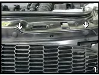
Using a flat screwdriver, remove two push pins on the top edge of the grille. Do this on both sides. Set push pins aside to be reinstalled later.
