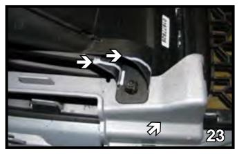
23. **2010 S Convertible:** On the back side of the fascia, using a utility knife trim along the top straight and out. Do this to both sides of the vehicle.
