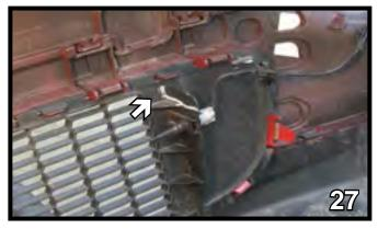
27. **2009 S Convertible:** Continuing on the back side of the fascia, using a utility knife trim down to the gusset and straight out (as shown). Do this on both sides.
