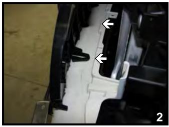
Remove the grille by pushing down.
