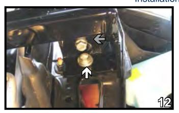
12. Remove the metric bolt (white arrow), replace bolt and washers with Loctite applied. Insert into the top hole (gray arrow) 3/8"-16 x 1-1/4' bolt with Loctite, 3/8" lock washer and tighten to 3/8"-16 nut plate. Then tighten the metric bolt. Do this on both sides.
