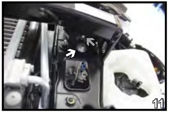
11. Hold the baseplate up in place and start the 8MM-1.25 x 50MM hex bolt (white arrow) with lock and two flat washers into existing hole, make it snug. Using the baseplate as a template, drill the hole above (gray arrow) with a 13/32" drill bit. Do this to both sides.
