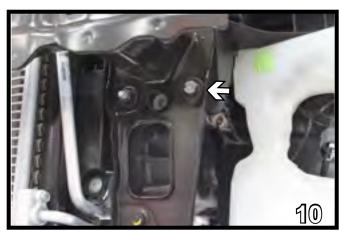
Under the reinforcement bumper, use the reciprocating saw to cut the outer bolt off so it is flush with the nut. Do this on both sides.
