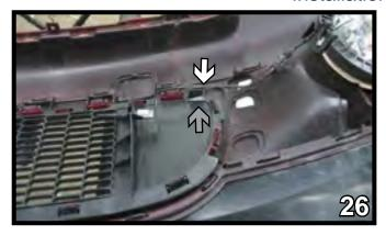
26. **2009 S Convertible:** On the back side of the fascia, passenger side, pull up the sensor. Using a utility knife, cut off the tab (gray arrow).
