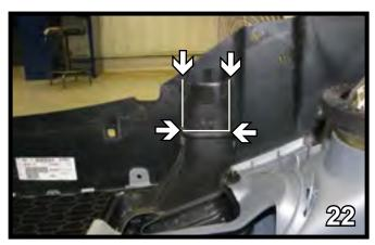
22. **2010 S Convertible:** On the back side of the fascia, using a utility knife trim down and across the bottom. Do this on both sides of the vehicle.
