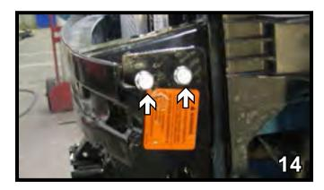
14. Into the holes drilled in the side also insert 3/8"-16 x 1-1/4" bolts with Loctite, 3/8" lock washers and 3/8" nut plates. Do this on both sides.
