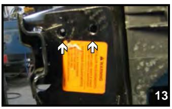
13. Using the baseplate as a template, drill two holes on the side. Do this on both sides using a 13/32" drill bit.
