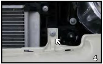
4. After removing the grille in front, remove the T25 Torx bolt. One on each side. Set bolts aside for later reinstallation.
