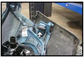
Located on both sides behind the grill, there is a temperature sensor that will need to be unplugged.
