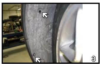
Forward of the front tire, use a flat screwdriver to remove two push pins. Do this to both sides. Set push pins aside for later reinstallation.
