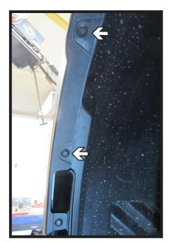
3. Remove the top two (2) push pins from along the edge of the wheel well. Do this on both sides of the vehicle.
