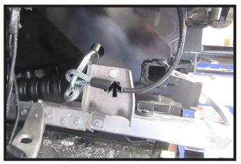
17. Reattach side bracket to frame by starting the bottom rear bolt (white) and the bottom front bolt (gray). Then using the hole from the baseplate as a guide drill a 3/8" hole (black) into the bracket and secure bracket to baseplate using 3/8" hardware. Do this on both sides of the vehicle.
