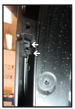
4. Release the two (2) clips from the back side of the fascia in the wheel well to start removing fascia. Do this on both sides of the vehicle.
