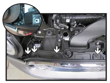
Using a T30 Torx, remove the eight (8) bolts from the top edge of the fascia.
