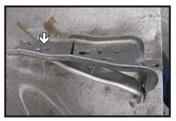
15. Using a T30 Torx, remove the bolt holding the secondary bracket to the primary bracket. Do this for both side brackets.
