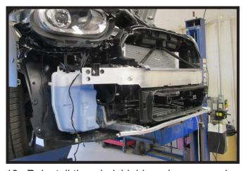
Reinstall the windshield washer reservoir and grill shroud.
