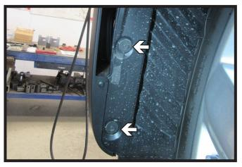
2. Using an 8MM socket remove the two (2) bolts from along the edge of the wheel well. Do this on both sides of the vehicle.
