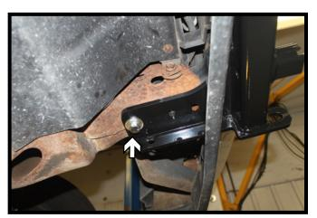
3. Position the baseplate onto the frame, aligning to the holes in the frame and clamp in place. Install a 1/2"-13 x 1-3/4" bolt with 1/2" lock and flat washers into the rear hole and a 1/2"-13 nut plate on the inside of the frame. Do this on both sides of the vehicle. Fully tighten all hardware.
