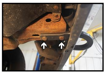
1. Using a 18MM socket, remove the four (4) bolts from the tow hooks. There are two (2) on each side.
