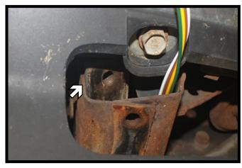
Remove the existing nut plates from the tow hook pockets.
