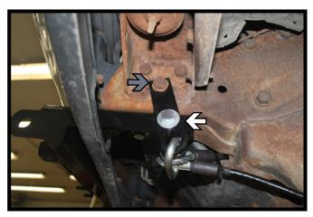
5. Using a 19MM socket, remove the existing bolt from the outside of the frame (gray). Install the safety cable bracket onto the frame, reusing the existing bolt and a 1/2"-13 x 1-3/4" bolt with 1/2" lock and flat washers (white) into the baseplate hole and a 1/2"-13 hex nut on the inside of the baseplate. Do this on both sides of the vehicle. Fully tighten all hardware.
