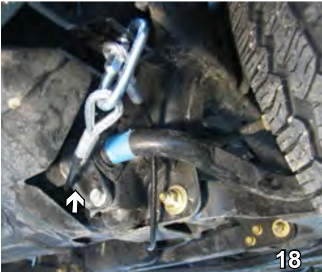
18. Attach the permanent baseplate safety cables to the provided convenience link on the baseplate. The photo above shows the recommended installation of the cables to frame of vehicle (see white arrow). Additional options may interfere with suggested mounting; in this case secure the cables to a solid piece of the frame as described in the instructions included with the permanent baseplate safety cables. Be sure the safety cables do not rub against any hoses or moving parts. Do this to both sides of the vehicle.
