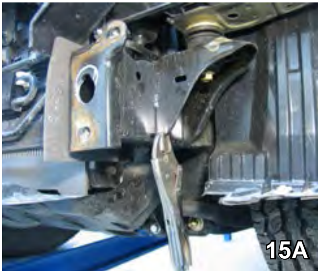
15. Using the vise grip bend the frame support, approximately 1/2" up from the bottom, back and fourth until it snaps off on both the front and back supports. Do this on both sides. (15A) On 2011-12 Models: In addition to front and back supports, snap off the area in front of the supports for additional baseplate clearance. Do this on both sides (15B)
