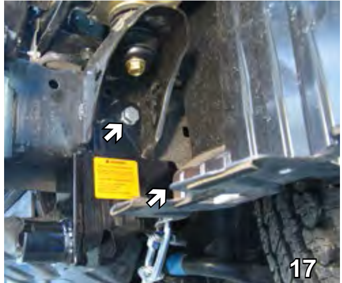
17. Insert the nut plate into the drilled hole on the frame cap to align with the drilled hole, tighten the 1/2"-13 hex bolt and 1/2" lock washer into the drilled hole. Repeat on other side. Be sure and use Loctite Red on all bolts before tightening.
