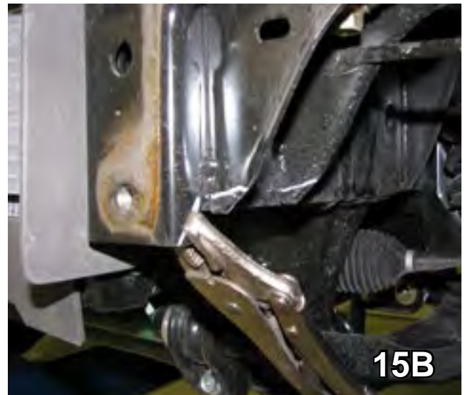
15. Using the vise grip bend the frame support, approximately 1/2" up from the bottom, back and fourth until it snaps off on both the front and back supports. Do this on both sides. (15A) On 2011-12 Models: In addition to front and back supports, snap off the area in front of the supports for additional baseplate clearance. Do this on both sides (15B)
