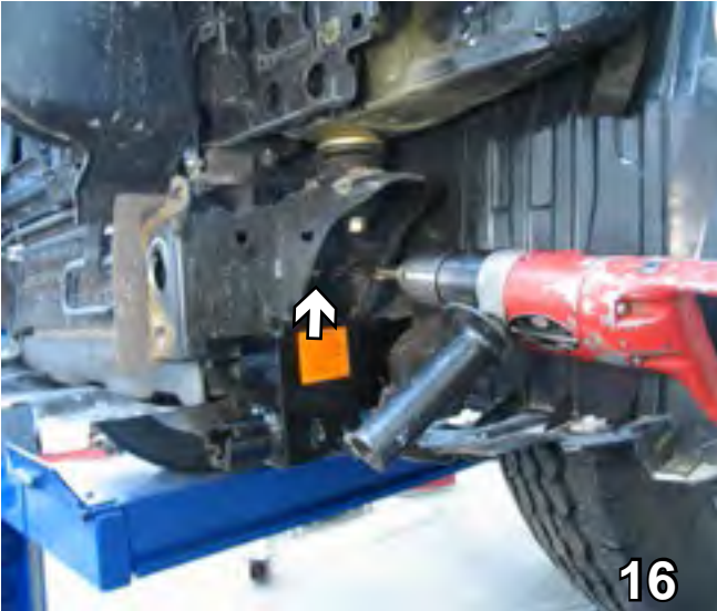
16. Using the baseplate as a template, drill a hole into the side of the frame rail with the 17/32" drill bit. Do this on both sides.
