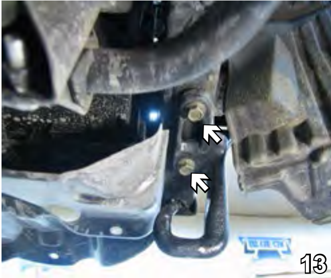
13. Remove the two (2) metric bolts from the tow hook on the passenger's side only using the 17MM socket. The tow hook will NOT be reinstalled.
