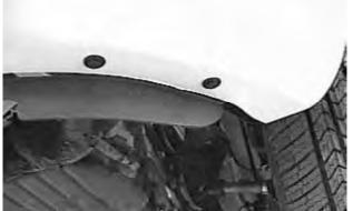
Remove the push pins from the bottom of the bumper fascia. Pull off the bumper fascia from the vehicle and set aside. Remove the rock guard connected to the lower cross member.
