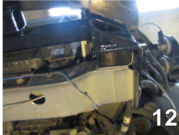
12. Drill 1 1/4" with hole saw into bottom of cross member. Do this to both sides.
