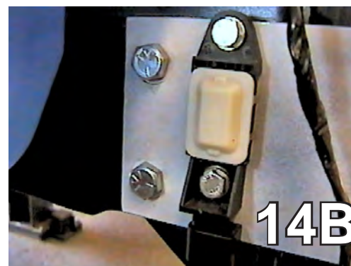
14. Using the diagonal cutters, cut off the alignment pin on the sensor and reinstall the sensor to its original position through obround
