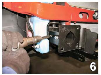
6. Using the baseplate as a template, drill the remaining three holes with the 17/32" drill bit. Do this to both sides of the vehicle.
