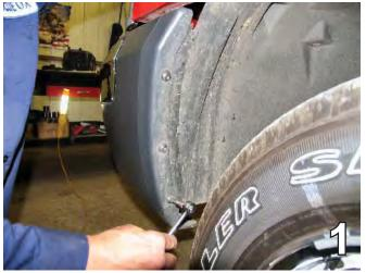
Using the 30 torx, remove three metric bolts from the edge of the wheel well, just forward of the front tire. Set the metric bolts aside to be reinstalled later. Do this to both sides of the vehicle.
