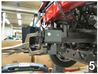
5. Slide the baseplate onto the frame rail to align forward side hole with existing hole in the frame and clamp in place with the vise grips. Do this to both sides of the vehicle. Insert the nutplate into the end of the frame rail to align with the existing hole, tighten the 1/2-13 x 1 1/2" hex bolt and lock washer with the 3/4" socket. Do this to both sides of the vehicle.
