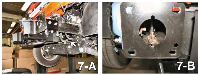
7. Insert the nut plates into the frame rail to align with the drilled holes, tighten the 1/2-13 x 1 1/2" hex bolts and the lock washer with the 3/4" socket into the nutplates. Do this to both sides of the vehicle.
