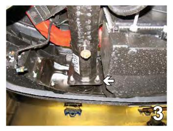
3. Using the 18MM socket, remove four metric nuts. Located just behind the metal bumper, on the frame end. Set the metric nuts aside to be reinstalled later. Pull the metal bumper forward, unplug the electrical connections and set the metal bumper aside to be reinstalled later.
