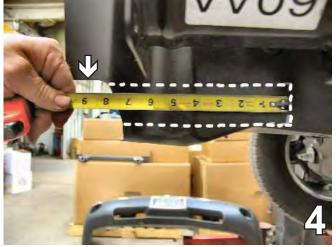
4. Measure and mark a horizontal line, 8" back from the lower front edge of the air dam, as indicated by the white arrow in the photo above, mark a horizontal line 2 1/2" below the first line and cut out the area with a utility knife. Do this to both sides of the vehicle. This will allow the baseplate to slide onto the frame rail.
