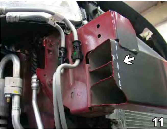
11. Using the reciprocating saw, cut the end of the bumper so that it is flush with the frame. Do this to both sides of the vehicle.
