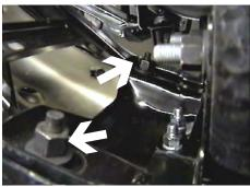
1. Using the 18MM socket, remove six metric nuts from the back side of metal bumper. Pull bumper forward, unplug electrical and set aside.
