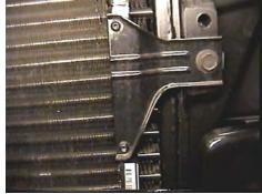
2. Remove metric bolt with the 13MM and two torx screw's with the 20 torx from radiator support on driver's side and set aside. Remove radiator bracket on passenger's side to open area for tow hook removal.
