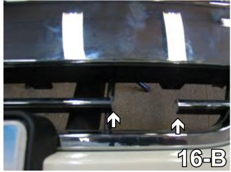
16. Using a utility knife, cut the fascia horizontal bar starting at the outer vertical bar and 3-1/2" out toward the edge. Do this on both sides of the fascia.
