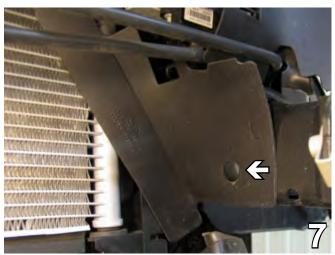
Remove the Christmas tree pushpin from the frame rail. Remove the air dam. Air dam will **NOT** be reinstalled. Do this to both sides of the vehicle.
