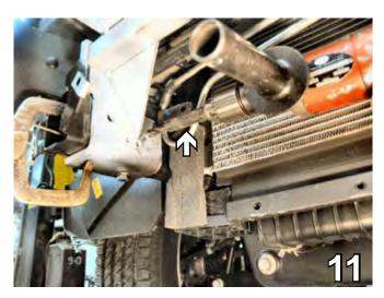
11. Using the baseplate as a template, drill the two (2) holes in the side of the frame rail with the 17/32" drill bit. Do this to both sides of the vehicle. Protect coolant pipe line when drilling (note the section of pipe on the drill bit).
