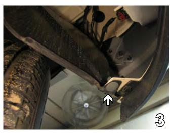
Just forward of the front tire on the fascia's lower edge, remove one (1) Christmas tree pushpin. Do this to both sides of the vehicle. Set pushpins aside to reinstall later.
