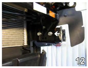
12. Insert the 1/2"-13 whiz nuts to align with the drilled holes inside the frame rail and tighten the 1/2"-13 x 1-3/4" hex bolts and 1/2" lock washers. Do this to both sides of the vehicle. Cut nut plate wires to make them flush with the end of the frame rail. This prepares the area for the metal bumper reinstallation.
