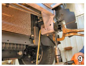
9. Slide baseplate between frame rails. Then slide baseplate forward just behind weld of the bumper bracket. Using vise grips, clamp in place to the bottom of the frame rail. Do this to both sides of the vehicle. Using the baseplate as a template, drill the two (2) bottom holes into the frame rail with the 17/32" drill bit. Do this on both sides of the vehicle.
