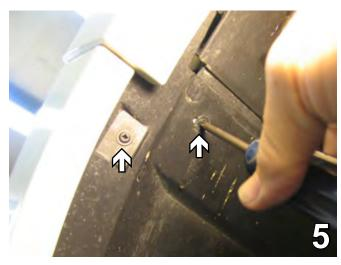
5. Just forward of the front tire on the fascia's corner, remove the two (2) screws with a Phillips screwdriver. Do this on both sides of the vehicle. Pull fascia corners down, then forward to release. Disconnect electrical connections. Set the fascia and screws aside to be reinstalled later.
