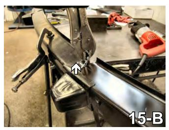
15. Secure the metal bumper to a work bench with the vise grips and cut designated areas from the previous step with the reciprocating saw. After cutting, clamp vise grip to the cut portion to be removed and move vise grip back and forth until cut portion breaks. Reinstall metal bumper to verify enough of metal bumper is removed. Trim as needed and reinstall bumper with existing hardware.
