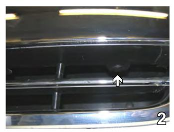
Remove the four (4) pushpins from upper fascia opening just behind the license plate bracket. Do this to both sides of the vehicle. Set pushpins aside to be reinstalled later.
