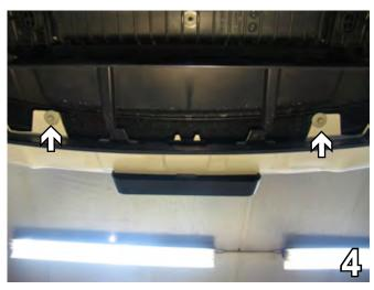
Using a 10MM socket, remove the two (2) metric bolts from lower tabs on the bottom edge of the fascia. Set the bolts aside to be reinstalled later.
