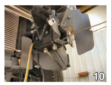
10. Insert the 1/2"-13 whiz nuts through the frame rail opening and align with the drilled holes. Insert the 1/2"-13 x 1-3/4" hex bolts and 1/2" lock washers and tighten. Do this to both sides of the vehicle.
