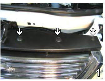
Using a Phillips screwdriver, remove three
