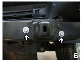
Using the 15MM socket, remove the two (2) metric bolts from the front of the metal bumper. Do this to both sides of the vehicle. Push down hard and out then pull the bumper forward. Set the bumper and metric bolts aside to be reinstalled later.
