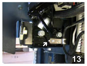
13. Insert the bent end of coolant bracket into the smaller front hole provided in baseplate on the passenger's side. Drill the self drilling screw in bracket hole provided in baseplate and into frame.
