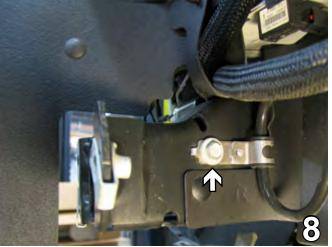
8. Using the 13MM socket, remove the metric bolt from the lower coolant line on the passenger's side, as indicated by the white arrow in the photo above. Some models may have a Block Heater cord bracket in this area to remove, as indicated by the grey arrow in the photo above.
